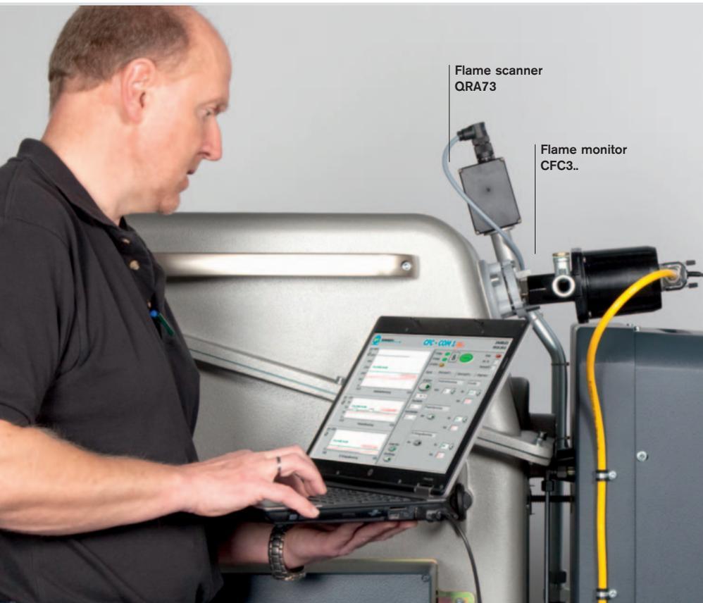
Testing and optimization via PC-Software Tool
